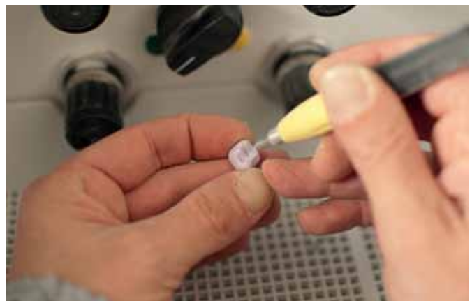
Fig. 5: At a pressure of 2 to 3 bar, fissures are tightened with focused blasting, and cusp elements are blasted out. As the abrasive of the quattro IS is dosed very precisely and has no lead and follow-up times, the material can be removed systematically. The special light in the sandblasting chamber (part of Renfert's "PerfectView" system) and the reduced dust development renders a clear view of the object.
